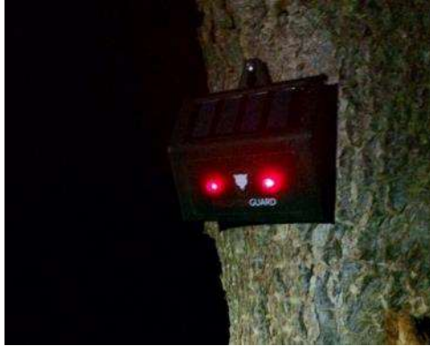
Solar powered flashing lights that look like eyes and deter predators and elephants
